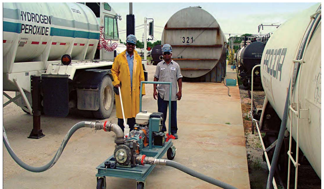
Operators at this chemical distribution/storage terminal facility transloading hydrogen peroxide from a railcar
